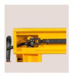
Unique push rod design helps in easy adjustment of forks for better stability
